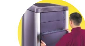
Easy expansion and increased system flexibility are offered by the Origin 200 GIGAchannel system, incorporating an additional five XIO slots and providing four PCI slots [seven total].
